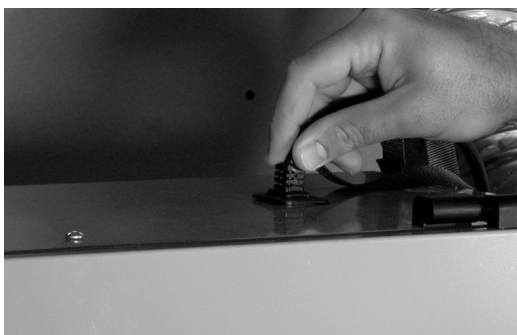
figure 10.1 Insert the power cord on top of the unit. Press firmly to make sure the power cord is secure.
